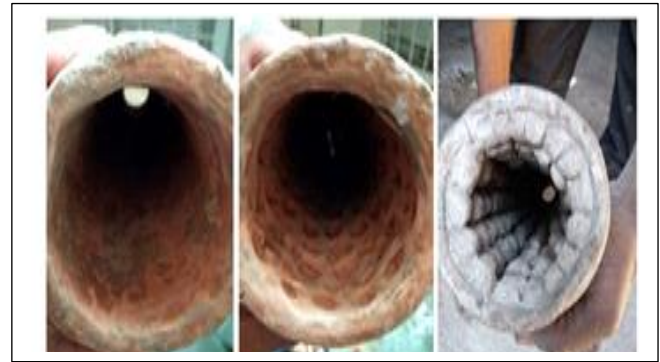
Fig. 1. Test Tubes (a) Plain Tube, (b) Dimpled Tube, (c) Protrusion Tube
