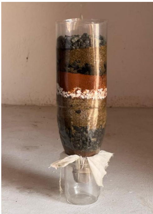
Fig. 6. Table-top Model of Natural Permeable Reactive Barrier
