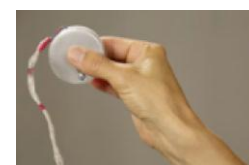
Figure 1: The grip force sensor.
