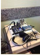
Figure 2: The portable device. We can see the grip force sensors, the amplifiers Honeywell DV10L, the data acquisition card measurement computing usb-1608GX and the headphone. The sound console is use in a other project.
