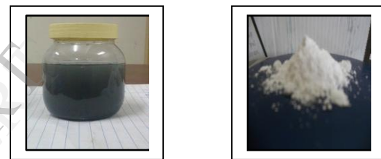
Figure 2 (c):- 1% volume concentration of (Al 2 O 3 – CuO/ H 2 O) Hybrid Nanofluid,(d) Aluminum oxide nanopowder
