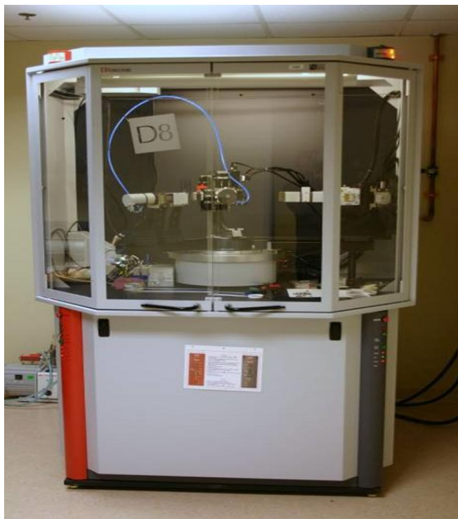
Fig-1 Bruker AXS D8 Discover XRD at NCAT, ) is used for identification of phases and crystallographic analysis of coatings , using high angle diffraction geometry Ref[5]
