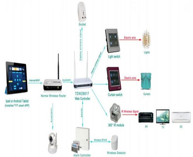
Figure 4: Wireless system (Source: Zygbee Home Automation)
