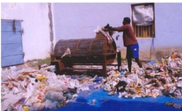
Figure 2: Cleaning and drying plastic waste
