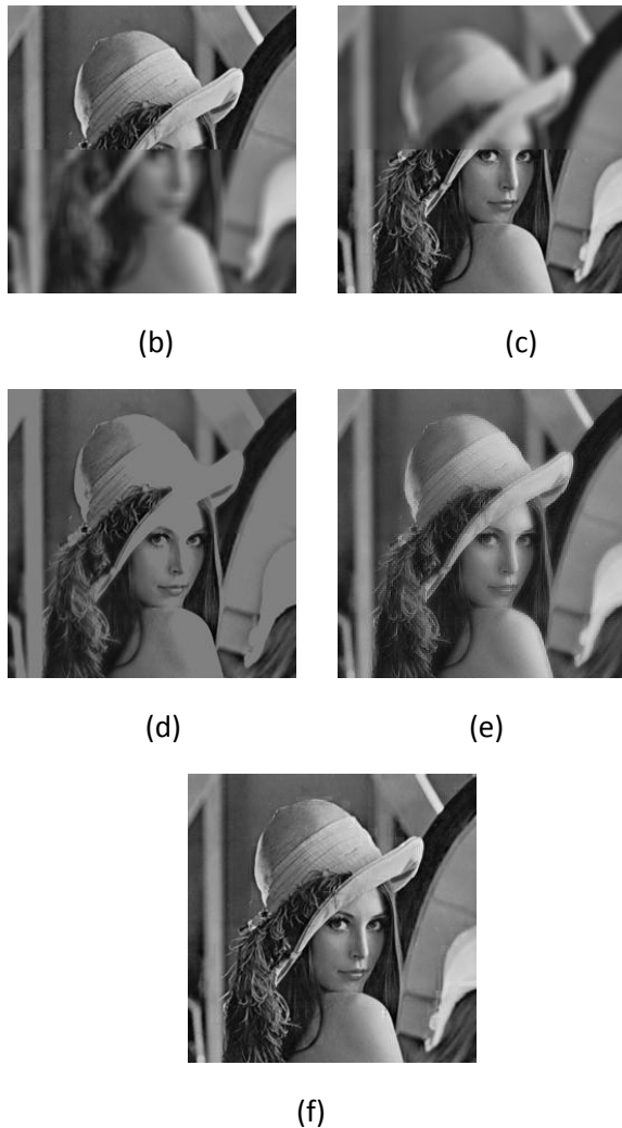
Figure 2. Simulation results of Lena images. (a) reference Lena image (b) Lena image blurred on the horizontal lower; (c) Lena image blurred on the horizontal upper; (d) fused image by pixel averaging method; (e) fused image by wavelet based mean-max algorithm; (f) fused image by proposed method using 5 level wavelet decomposition;
