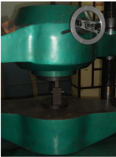
Figure: 5 Universal testing machine with shackles and specimen fitted
