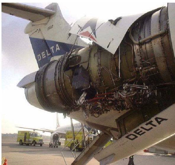
Figure: 2 Engine Failure seen during blade-off event
