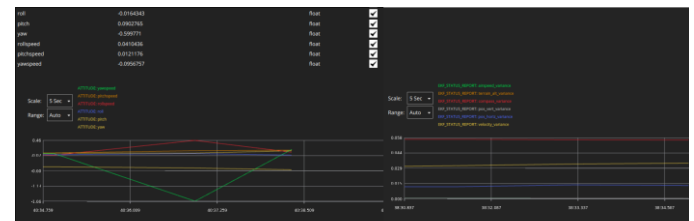
Fig 5. a) Attitude Yaw, Pitch, Roll of drone while using OA method b) EKF 2 status report of drone in different variance
