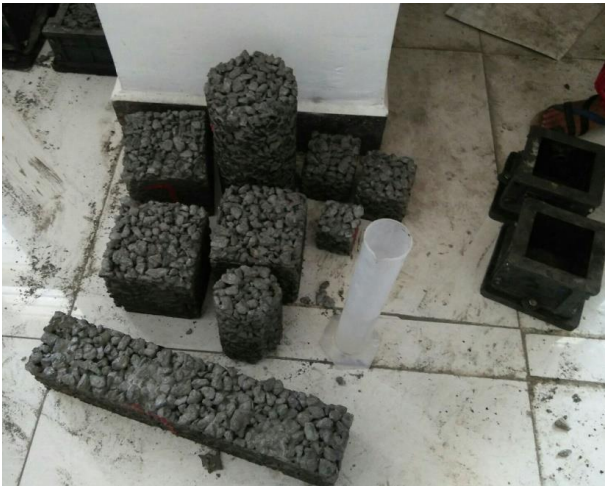
Compressive Strength Test Results Samples prepared using cement and coarse aggregate
