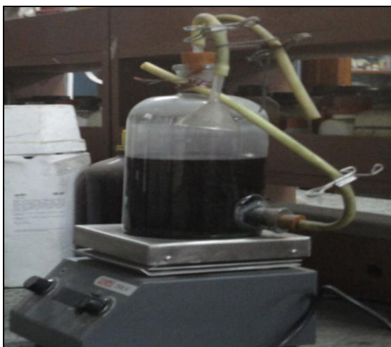
Fig.-2: Experimental Setup of Batch Reactor for Denitrification Study
