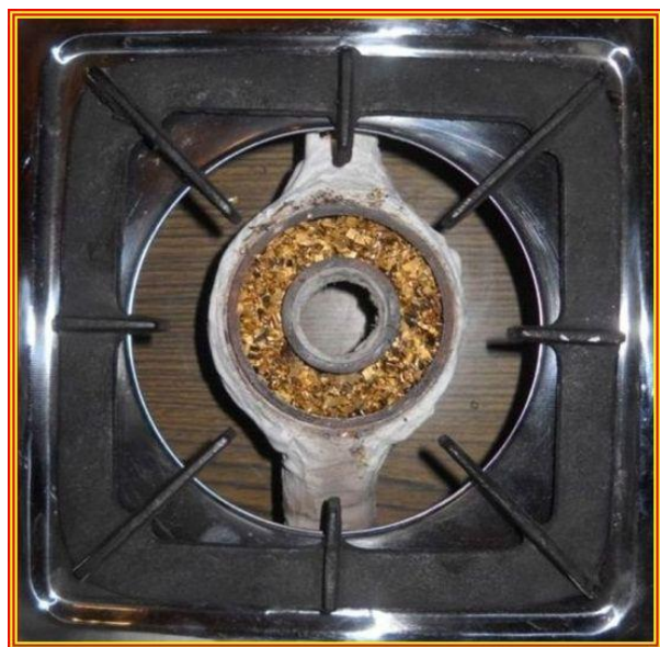
Figure 3 Insulated LPG stove filled with brass chips
