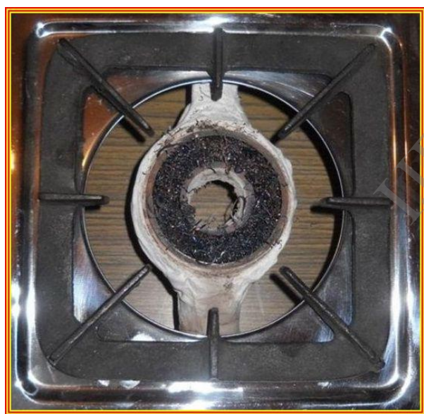
Figure 4 Insulated LPG stove filled with mild steel chips
