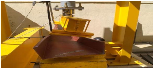
Plate 4. Buckling of steel outwards and bending
