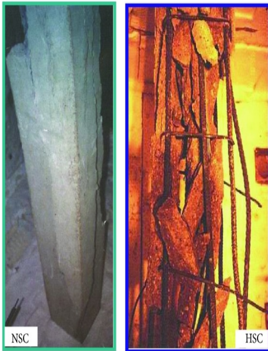
Fig. 5: Fire induced Spalling in 1) Normal strength concrete 2) High strength concrete [15]
