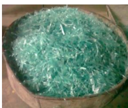
Fig.1: Hand cut fibres
