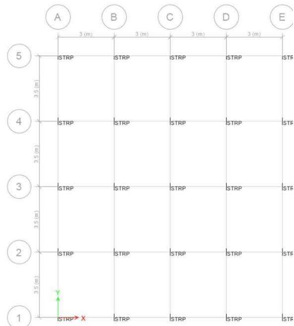
Fig.4 Plan and isometric view of G+5 RC building with STRP pads
