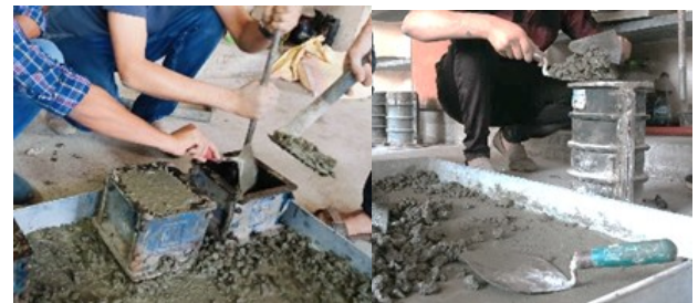
Fig. 2. Concrete was filled into mould
