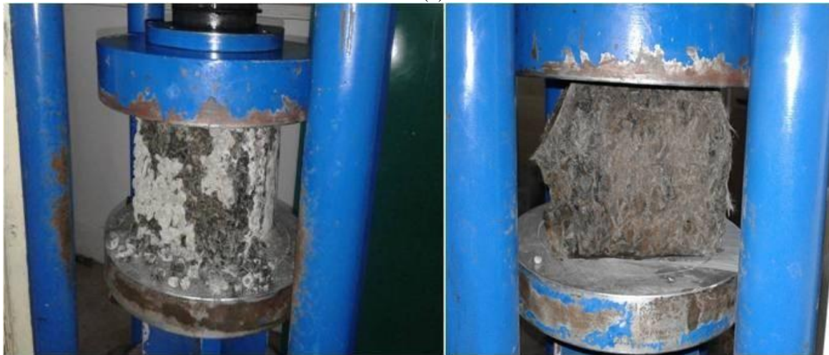
Pic (b)- shows the permeable concrete cube during compressive strength test.
