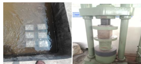
Fig. 9 Curing and testing of compressive strength
