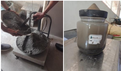
Fig 5 Specific gravity test for cement
