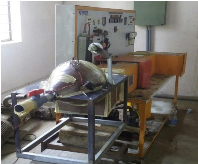
Fig.3. Dehumidifier connected to the air conditioning unit
