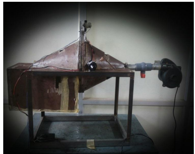
Fig.2. Designed composite solid desiccant wheel dehumidifier
