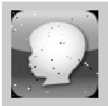
Figure 14: Reconstructed image using Median Filter
