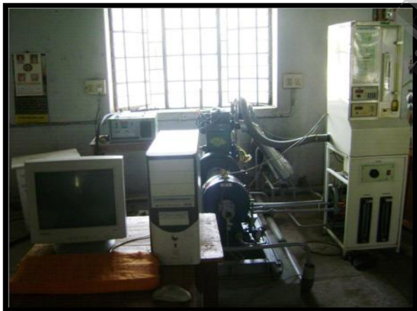
Fig.01 Experimental setup diagram of Diesel Engine
