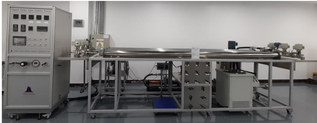
Figure 1. Pipeline Friction Loop System
