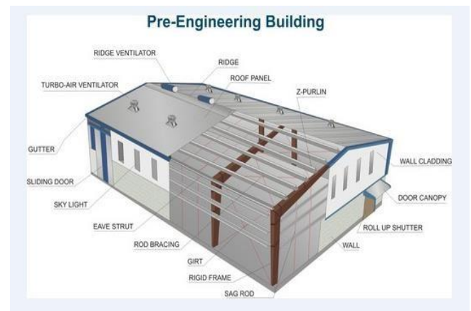
Fig 1: Pre Engineered Building Parameters.
