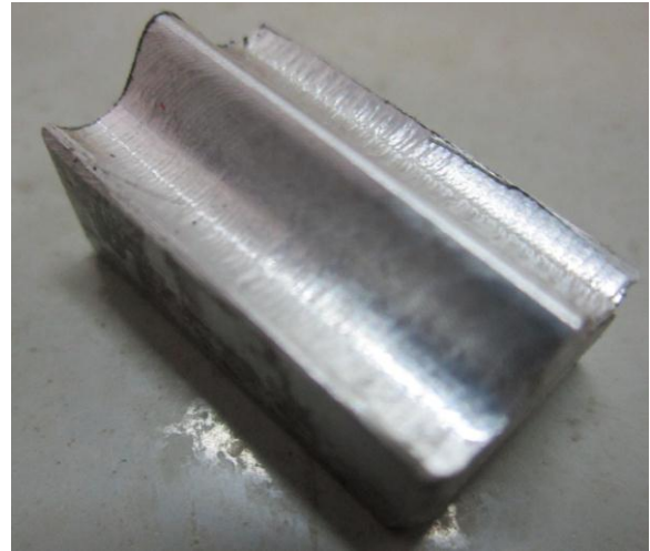
Fig. 1. Free-form surface after ball-nose finishing.
