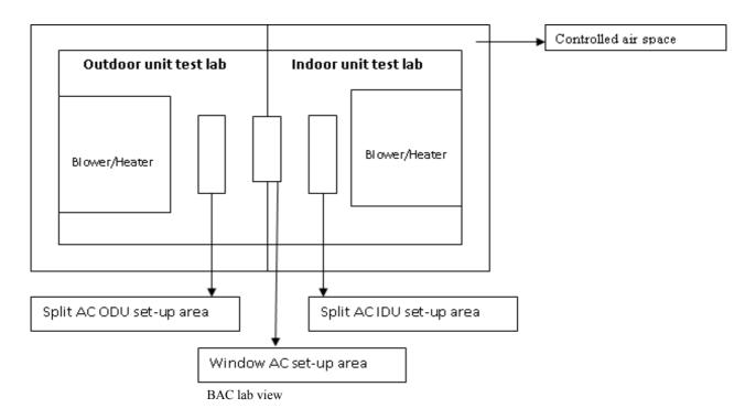
Each test room consists of the following equipment
