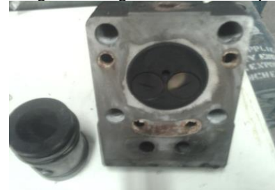
Fig.3.1. Zirconium Oxide coated piston
