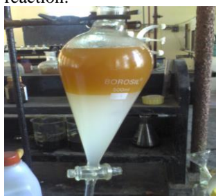
Water wash and separation of biodiesel from water
