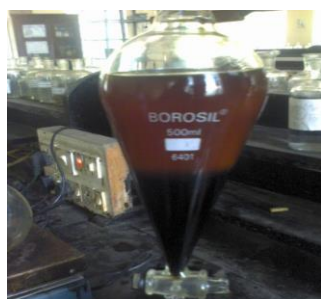
Separation of glycerine from biodiesel
