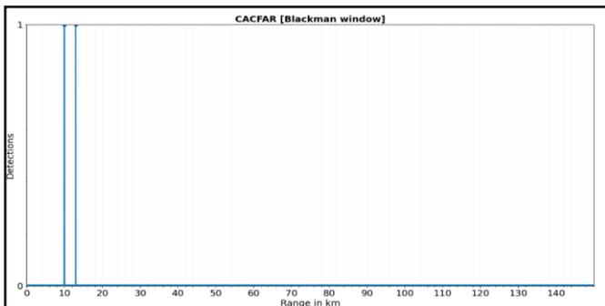
Fig 11 : Target detections with Blackman window
