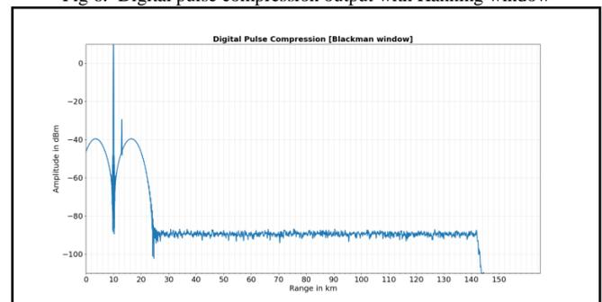
Fig 7 : Digital pulse compression output with Blackman window
