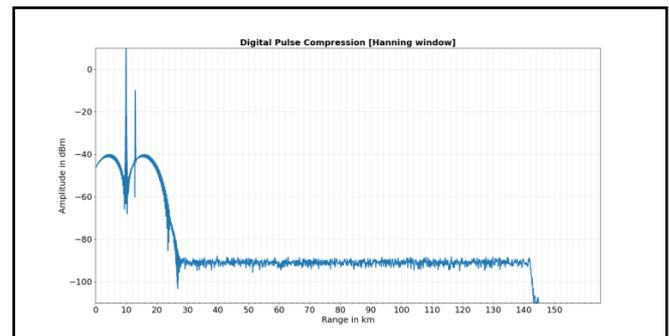
Fig 6: Digital pulse compression output with Hanning window
