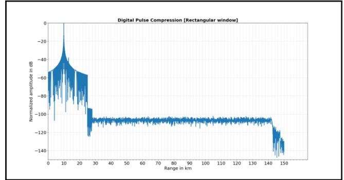
Fig 4 : Digital pulse compression output with Rectangular window
