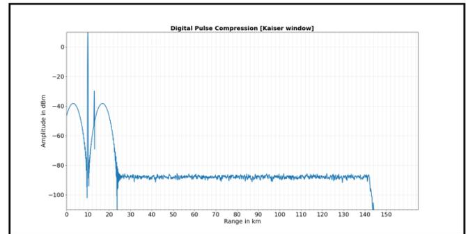
Fig 5: Digital pulse compression output with Kaiser window
