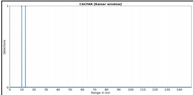
Fig 9 : Target detections with Kaiser window
