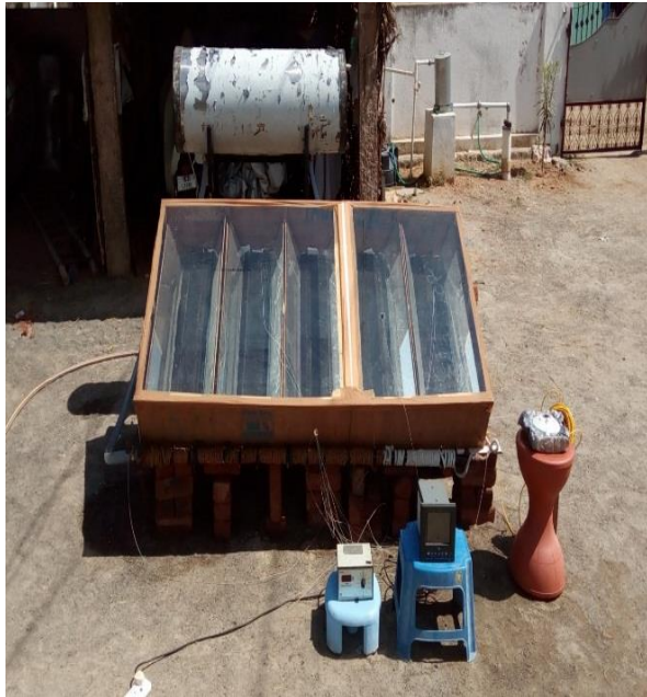
Fig.7. Photographic view of thermosyphon V-trough solar water heater.
