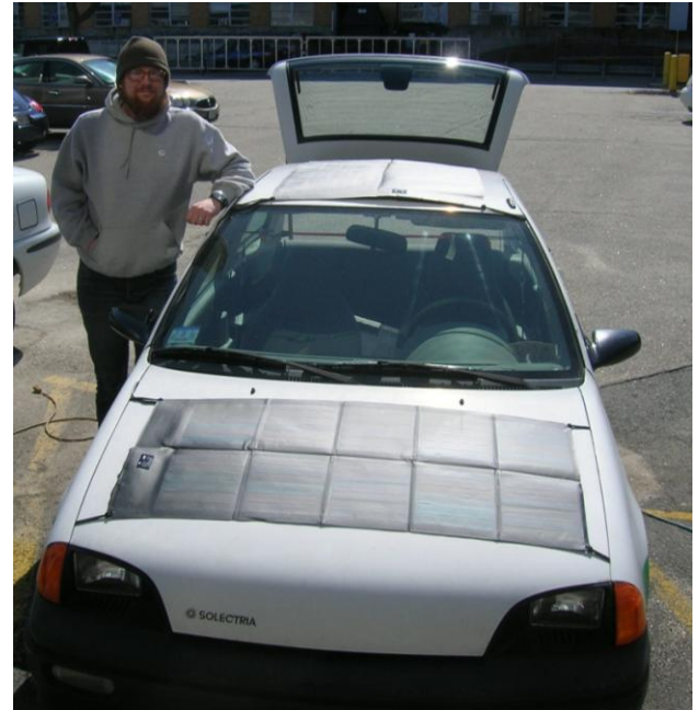
Fig. 2 Electric car with PV panels on the roof and the hood
