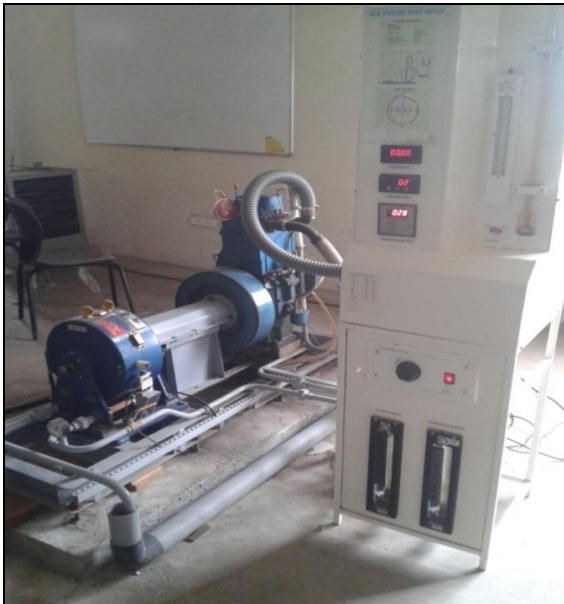
Fig No-2. 1 Experimental setup of VCR Engine
