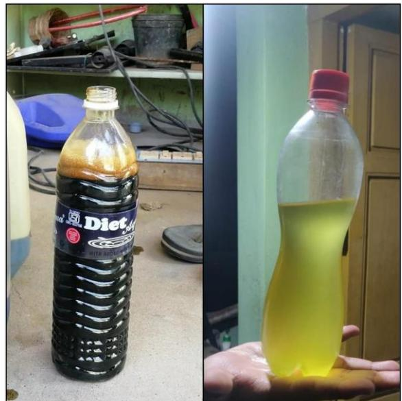
Fig 4.5 Raw plastic oil and Distilled plastic oil
