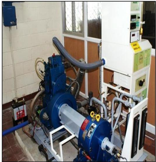
Fig 4.4 Kirloskar single cylinder four stroke diesel engine
