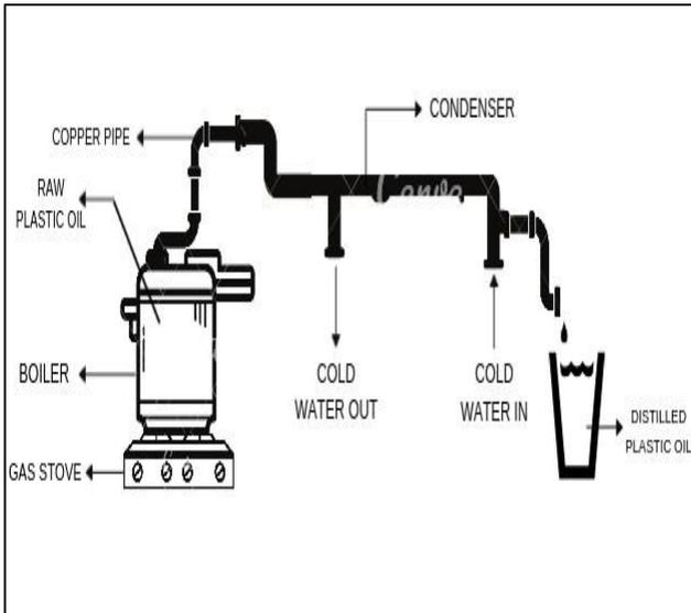
Fig 4.1 Design for distillation setup
