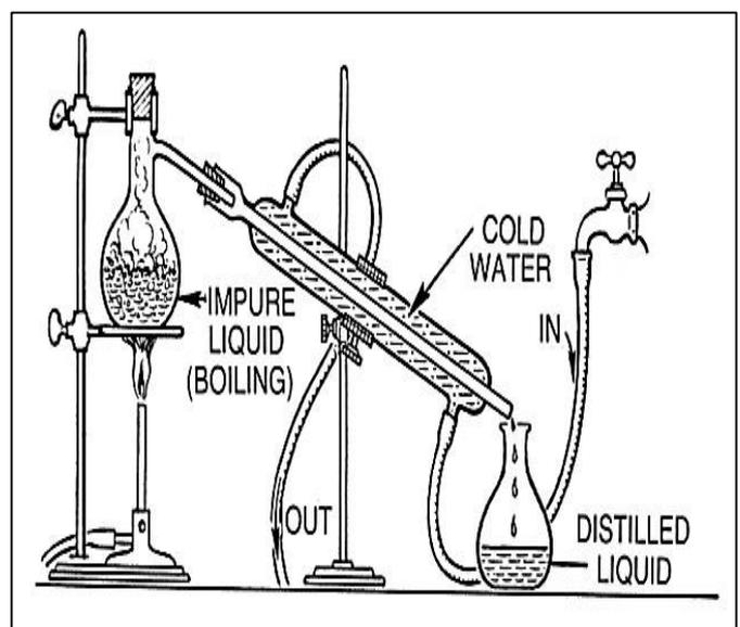
Fig 1.2 Distillation setup
