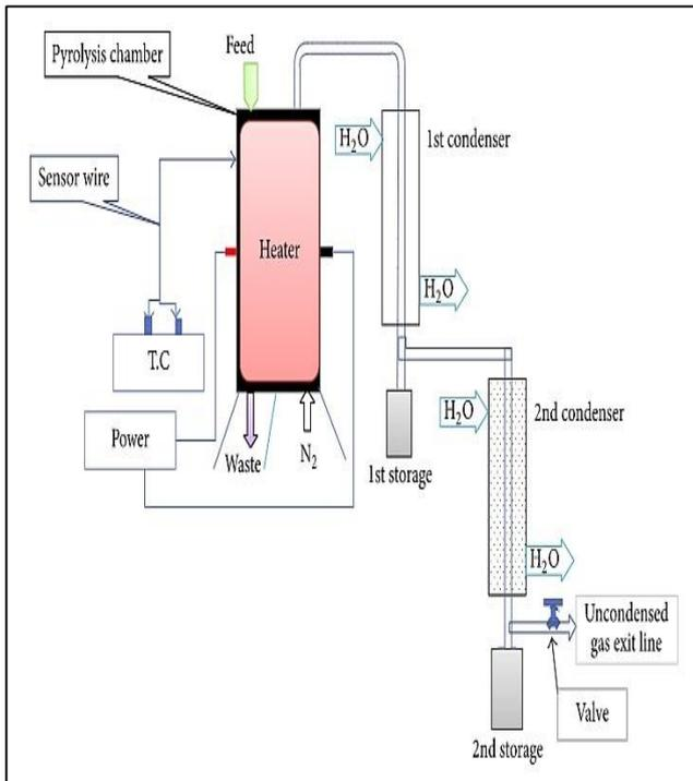
Fig 1.1 Schematic representation of plastic pyrolysis setup
