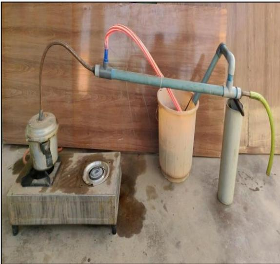
Fig 4.2 Distillation setup for plastic oil
