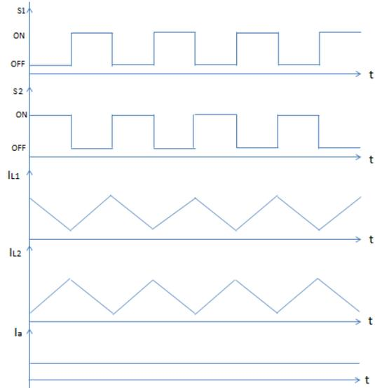
Fig 6.Voltage and current waveforms of IBC
