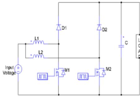
Fig 3.Circuit diagram of IBC Converter
