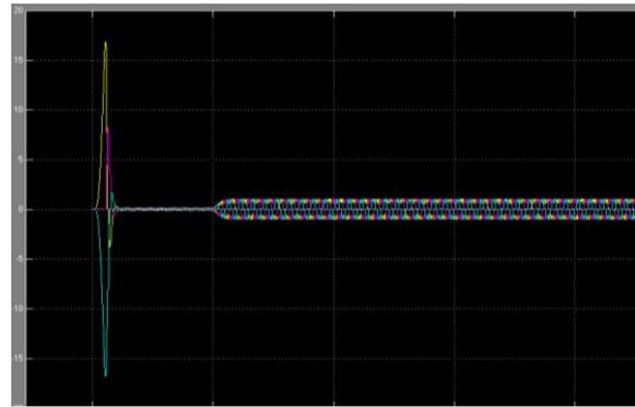
Fig 9. Rotor speed of Bldc motor
