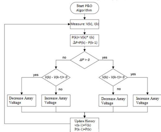
Fig 2. Flowchart of P&O algorithm
