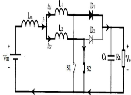
Fig 5.IBC mode 2 operation
