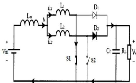
Fig 4.IBC mode 1 operation
