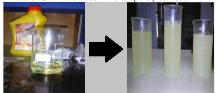
Fig. 4. Pure POE oil with Cu doped MgO Nanoparticles [0.2%, 0.4%, 0.6% vol.]
