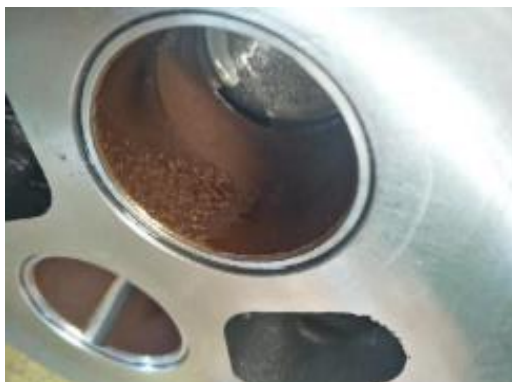
Figure 7 Failure morphology of the journal bearing
