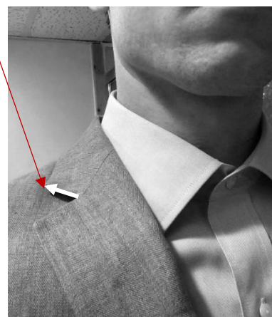
Fig.2a. Observed Collar point Pulling
