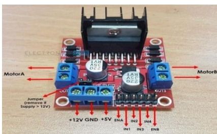
Figure 4: L298 Driver Module
