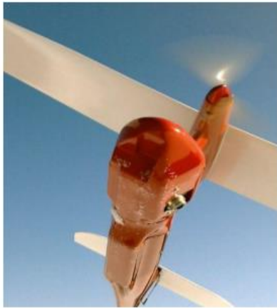
Figure 2: Pteryx UAV for aerial photography is an example of a UAV civilian application [8].
