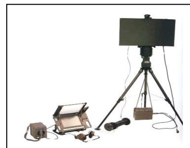
Fig 1: Battle Field Surveillance Radar (Short Range)
