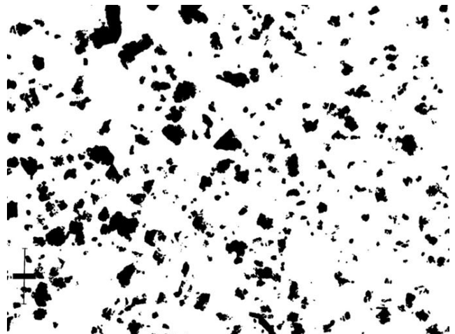
Fig. 5 After converting previous image in binary, filtration and segmentation using modified approach
