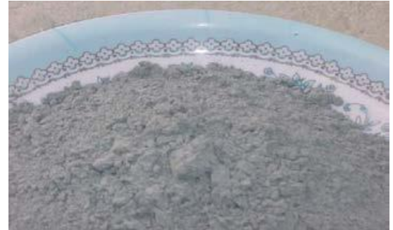
Figure 3.4 . Sample of RHA after 1 hour of Grinding
