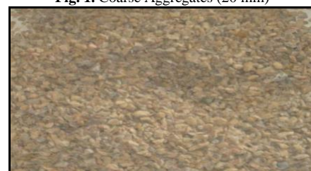
Fig. 2. Coarse Aggregates (10 mm)
