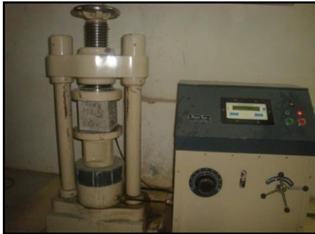
Figure.4.1 Compressive strength testing
