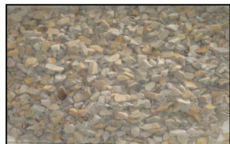
Fig. 1. Coarse Aggregates (20 mm)
