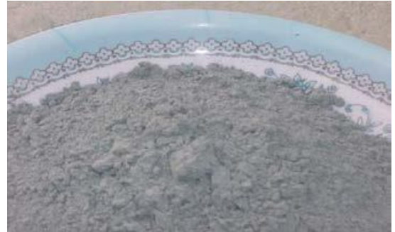
Figure 3.4 . Sample of RHA after 1 hour of Grinding
