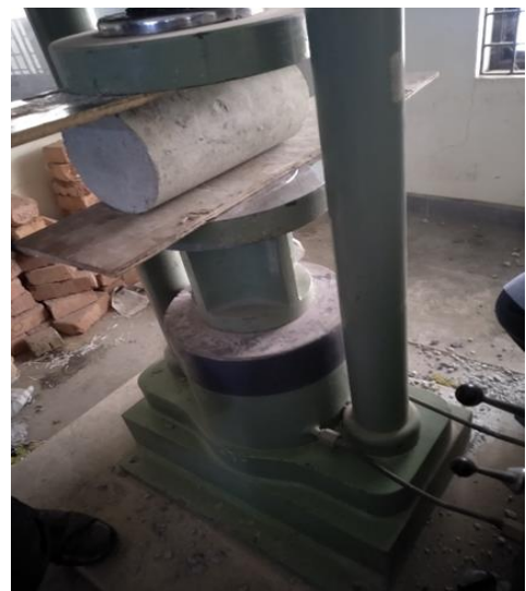
Fig. 9. Flexural Strength Test for Concrete Cylinder
