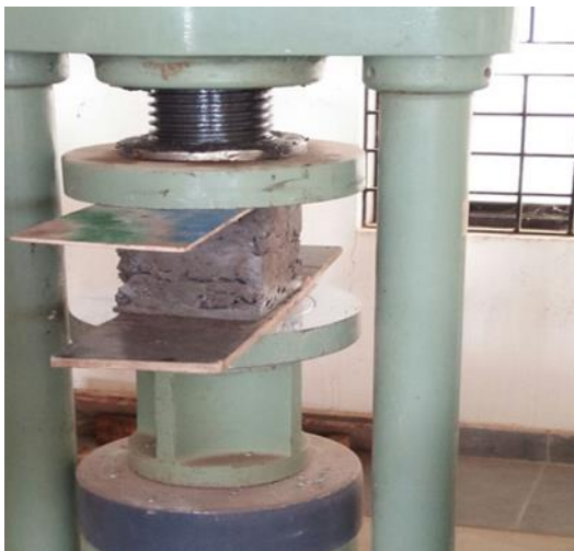
Fig. 7. Compressive Strength Test of Concrete Cube
