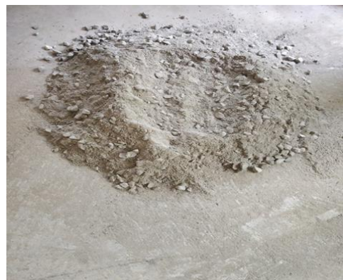
Fig. 3. Mixing Stage Before Addition of Water
