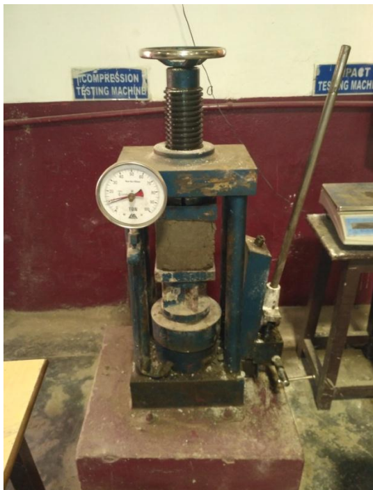
Fig. 2. Compressive testing machine.
