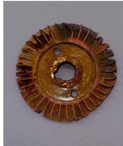
Fig.4 The damaged impeller
