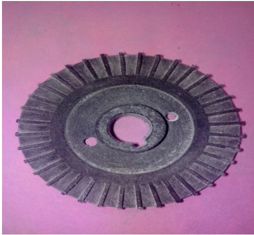
Fig.21 Rapid prototype of impeller
