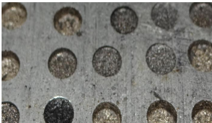
Figure 1: Work piece after removal of material
