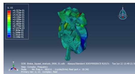
Fig.21 Mode shape at 44<sup>th</sup> Mode(case-2.1)
