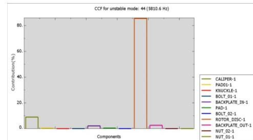
Fig.22 CCF for unstable mode: 44(5810.6 Hz)
