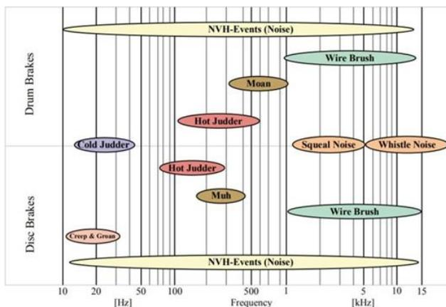
There are various kinds of brake noises and vibrations with numerous terminologies to nominate the phenomena in the literature that are probably inconsistent. One of the terminologies. Noises and vibrations can be classified that are based on frequency range. Some types of brake noise and vibration can be summarized.
