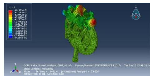
Fig.23 Mode shape at 54<sup>th</sup> Mode(case-2.2)
