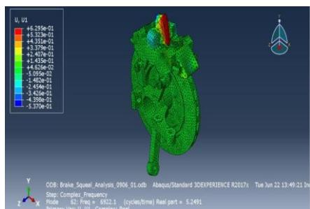
Fig.25 Mode shape at 62<sup>nd</sup> Mode(case-2.3)
