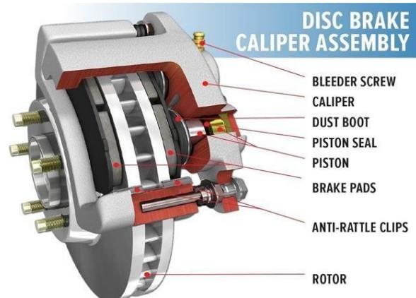
Fixed-caliper design, bolted solidly to the flange, has either two or four pistons which push the pads out. Fixed-caliper disc brakes have more balanced inner and outer pad wear with less pad taper than floating caliper designs. They require no anchor or integral knuckle for shoe support.
