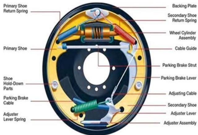
Automotive friction brakes are grouped according to their basic designs into two classes: Drum brakes use brake shoes that are pushed out in a radial direction against a brake drum. Disc brakes use pads that are pressed axially against a rotor or disc. Advantages of disc brakes over drum brakes have led to their universal use on passenger-car and light-truck front axles, many rear axles, and medium-weight trucks on both axles.
