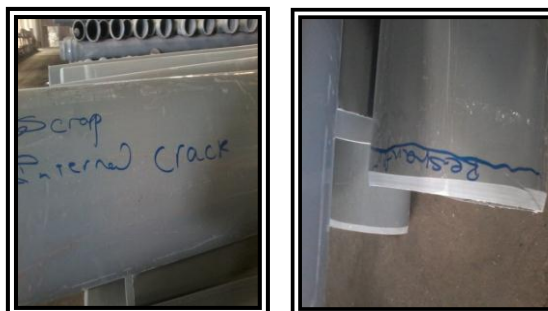
(3) Cracking (4) chamfering problem
