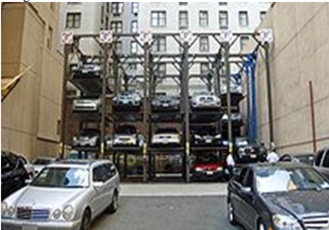
Multi level parking arrangement for cars
