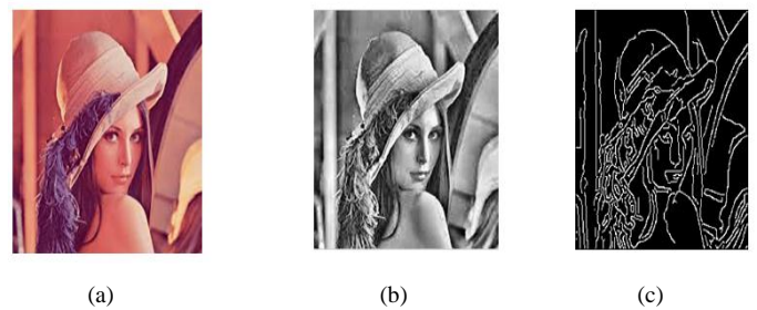
Fig.11 a) Original Lena image b) Enhanced gray scale image c) Equalized edge map
