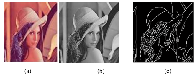
Fig. 10 .(a) Lena image (512 x 512) (b) Gray scale image (c) Canny edge map of original Lena image
